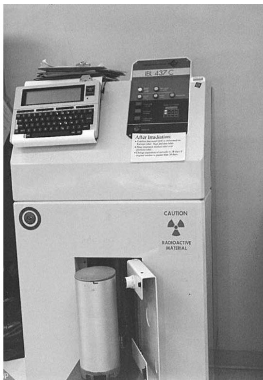
Figure 11–9. Irradiators are used to prevent lymphocytes in RBC products from causing graft-versus-host disease in susceptible patient populations. (Courtesy National Institutes of Health, Bethesda, MD.)
